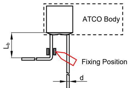
**TABLE YM-3** Distance between Body and Bending Point
